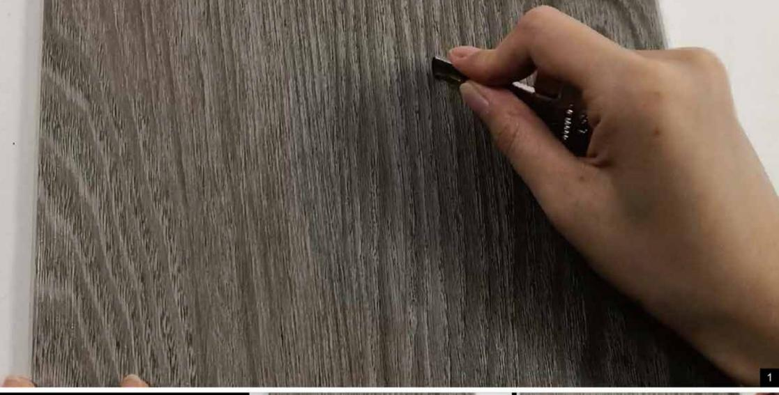
Finfloor manufacturers use "ceramic bead" technology, which is incorporated into the UV layer.
